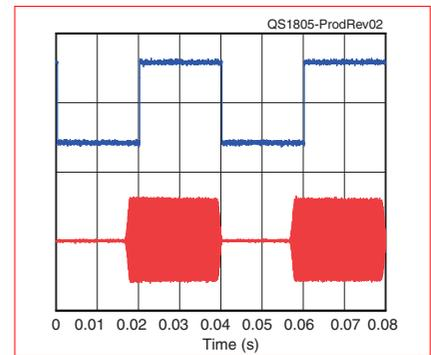
**Figure 2** — CW keying waveform for the Yaesu FT-991A showing the first two dits in full-break-in (QSK) mode using external keying. Equivalent keying speed is 60 WPM. The upper trace is the actual key closure; the lower trace is the RF envelope. (Note that the first key closure starts at the left edge of the figure.) Horizontal divisions are 10 milliseconds. The transceiver was being operated at 100 W output on the 14 MHz band.
