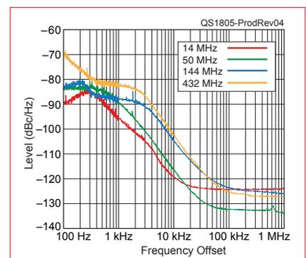
**Figure 4** — Spectral display of the Yaesu FT-991A transmitter output during phase-noise testing. Power output is 30 W on the 14 MHz band (red trace) and 50 MHz band (green trace), and 20 W on the 144 MHz (blue trace) and 432 MHz (yellow trace) bands. The carrier, off the left edge of the plot, is not shown. This plot shows composite transmitted noise 100 Hz to 1 MHz from the carrier. The reference level is  $-60$  dBc/Hz, and the vertical scale is 10 dB per division.
