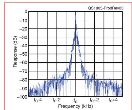
**Figure 3** — Spectral display of the Yaesu FT-991A transmitter during keying sideband testing. Equivalent keying speed is 60 WPM using external keying. Spectrum analyzer resolution bandwidth is 10 Hz, and the sweep time is 30 seconds. The transmitter was being operated at 100 W PEP output on the 14 MHz band, and this plot shows the transmitter output  $\pm 5$  kHz from the carrier. The reference level is 0 dBc, and the vertical scale is in dB.
